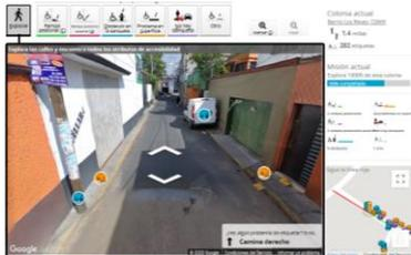
**Fig. 2:** The Project Sidewalk interface (in Spanish) showing narrow sidewalks with surface problems (orange labels) and physical obstacles (blue labels) in Azcapotzalco, MX. Screenshot from Twitter user @Gari01234.
